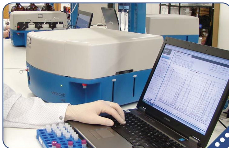
Figure 1. The Virus Counter instrument is a compact, bench top instrument with a footprint of 1.5 ft 2 (0.14 m 2 ).
